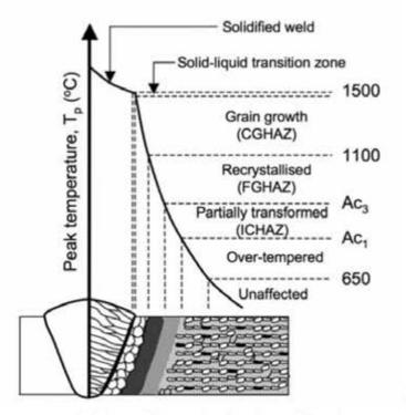
Schematic of welded ferritic alloys like Grade 91. Type IV cracking occurs in the FGHAZ region. Francis, et al, 2006, Mat. Sci. and Tech. Vol. 22 No. 12, pp. 1387-1395
